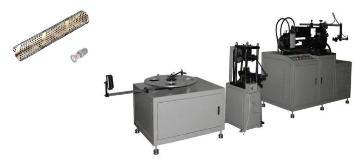
This machine is used to manufacture the center tube for the oil, fuel and hydraulic filters. It can produce the perforated or louvered holes.
