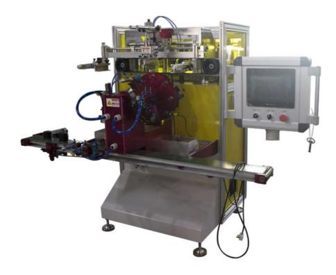
This machine is used to print the shell of the spin on filters.
