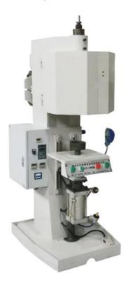
It is used for spin on oil fuel filter or other metal container sealing.
