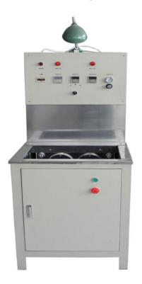
It is used for testing sealing performance of spin on filter.
