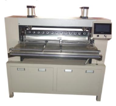
The knife pleating production line is used to pleat the filter paper,non-woven,active carbon etc, material for the auto filters industry.hydraulic filtration,purification and water treatment industries, etc.
