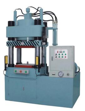
This machine is used to stretch the outer shell of the oil filter to increase the strength and durability of the shell.
