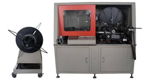
This machine is used to produce the inner and outer mesh forthe heavy duty air filters directly from the metal strip.
