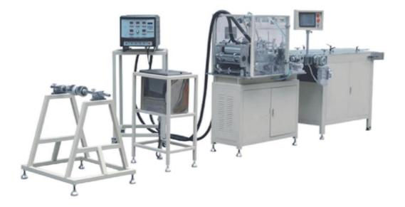
This paper pleating production line is used for making the panel air filter
